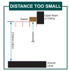
Add spacer to side of beam to achieve the optimum distance.
