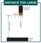
Add spacer under beam to achieve the optimum distance.
